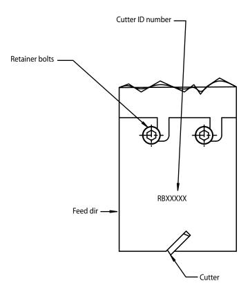
The proper cutter must be used that corresponds to the cavity to be abraded. Accurate abrading cannot be obtained without matching the proper cutter to the extrusion. Consult Azon for tooling recommendations.
